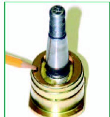
INSTALL INBOARD is stamped on the bottom of upper ball joint
