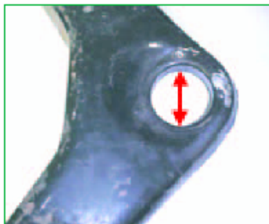
Check hole diameter for elongation
