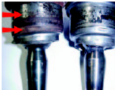
Inspect ball joint housing for excessive wear
