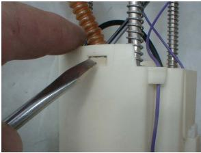
Depress the plastic tabs holding the module reservoir (bucket) on both sides, then slide the reservoir down and off the pump.
