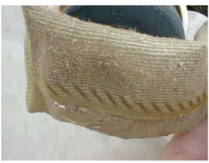
An inspection of the inlet filter to the pump may show a collection of "stuff" that can cause the filter to collapse thus restricting fuel flow, loss of volume and a reduction of pressure. Note; The secondary filter is finer than the primary sock.
