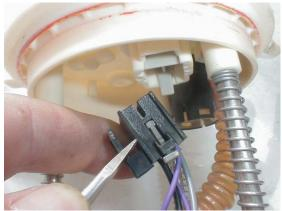
Remove the connector to the fuel pump and sender assembly
