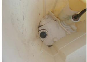
Inspect the inside bottom where the fuel pump lives. If there is debris, dirt, sand, etc., perhaps it is time to sell a tank cleaning or new tank. This becomes the fork in the road of the diagnostic path.
