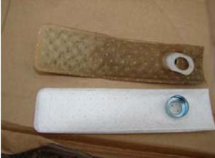
Remember to look for the answer inside the tank and fuel pump. Remember, the filters are white & clean when new as first installed. If dirty, the contamination came from somewhere.
