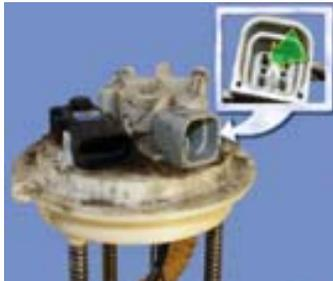
Excessive ethanol is a contaminate in systems that are not designed to operate with more than ASTM E-10. Fuel pumps that are designed to operate in a corrosive environment like ASTM E-85 are specially designed high-carbon content commutators.
